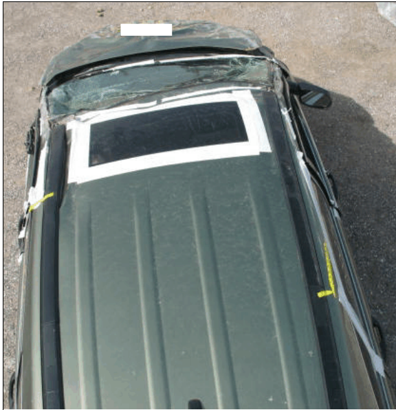
Figure 7: Damage to the top plane
