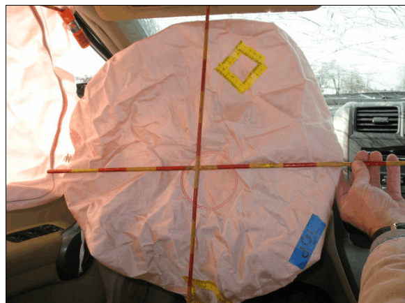
Figure 13: The driver's frontal air bag; each increment on measurement rods is 5 cm (2 in); steering wheel is rotated clockwise approximately 90 degrees
