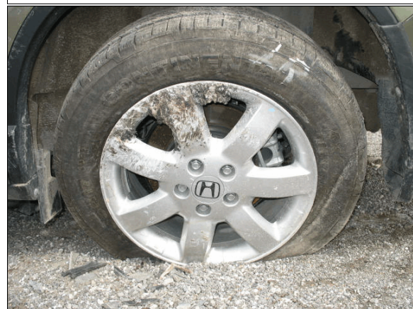
Figure 17: Damage to the Honda's left rear wheel
