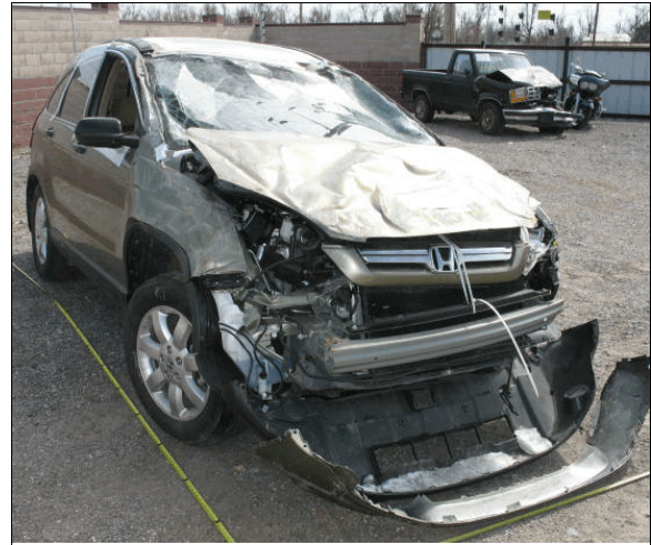
Figure 8: Damage to right side from the rollover
