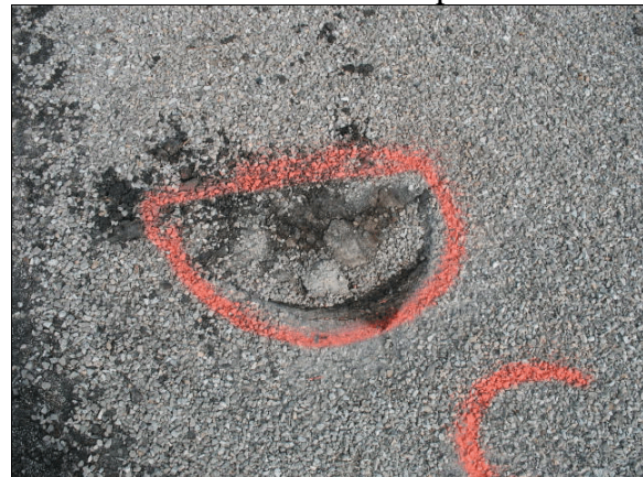
Figure 16: Gouge on the shoulder due to impact by the Honda's left rear wheel
