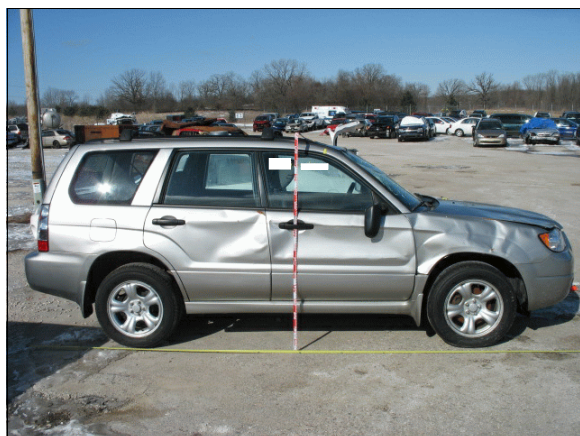
Figure 4: Right side damage
