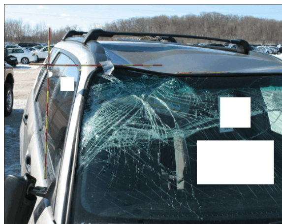
Figure 5: Subaru's maximum roof crush
