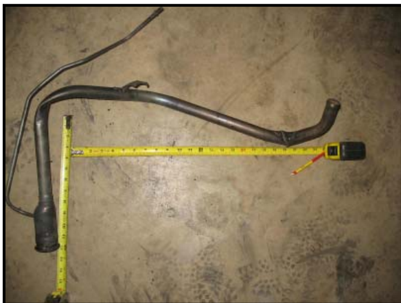
Figure 16: View of the deformed filler tube.
