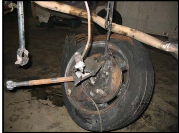
Figure 12: Damaged left rear wheel and suspension.
