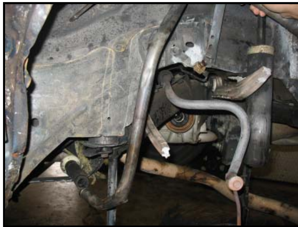
Figure 20: View of the separated inlet and filler tube reconstructed for reference.
