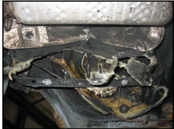
Figure 19: View of the burned tank looking to the left side of the Dodge.
