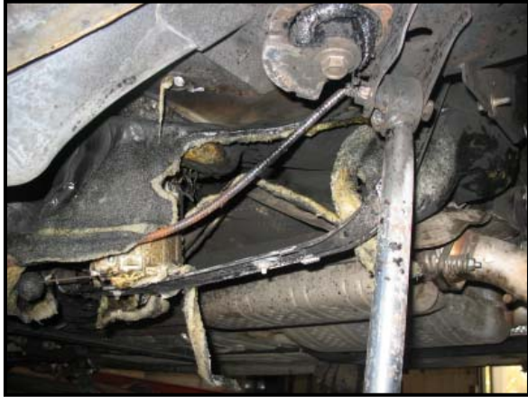
Figure 18: View of the burned tank looking to the right side of the Dodge.
