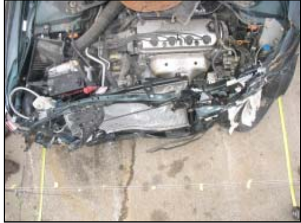
Figure 22: Overhead view of the frontal damage.
