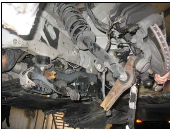
Figure 14: Front right suspension damage.
