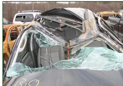
Figure 8. Roof crush, vertical and lateral.
