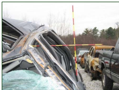
Figure 15. Lateral crush to the greenhouse area that created an ejection portal for the driver’s head.
