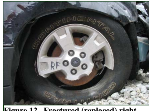
Figure 12. Fractured (replaced) right front alloy wheel and tire.
