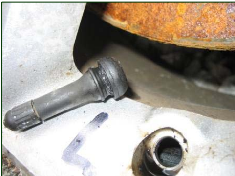
Figure 9. Removed LF valve stem.
