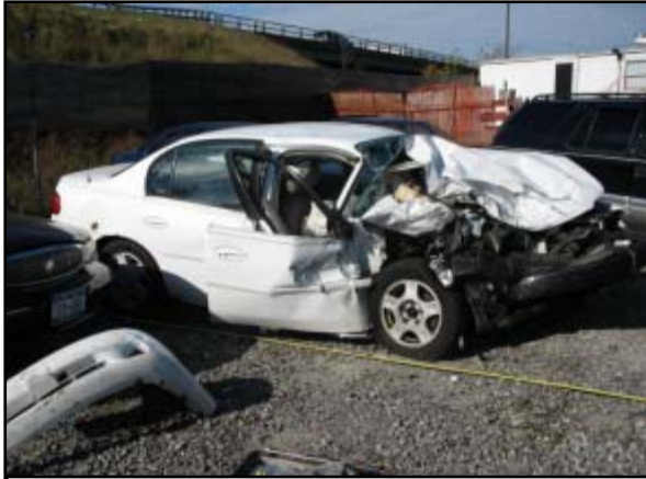
Figure 6. Front right view of the frontal damage to the Chevrolet .
