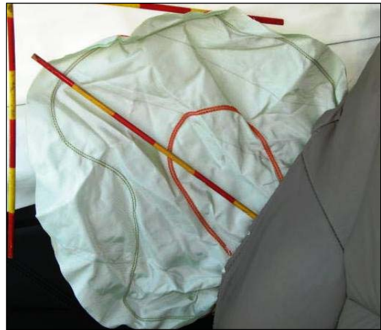
Figure 6: Deployed right seatback-mounted air bag.
