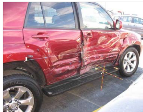
Figure 5: Right side damage pattern on the Toyota.
