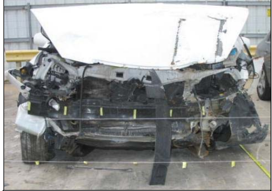
Figure 6: Frontal damage from barrier-type crash.
