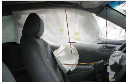
Figure 11: Deployed left side impact air bag system.
