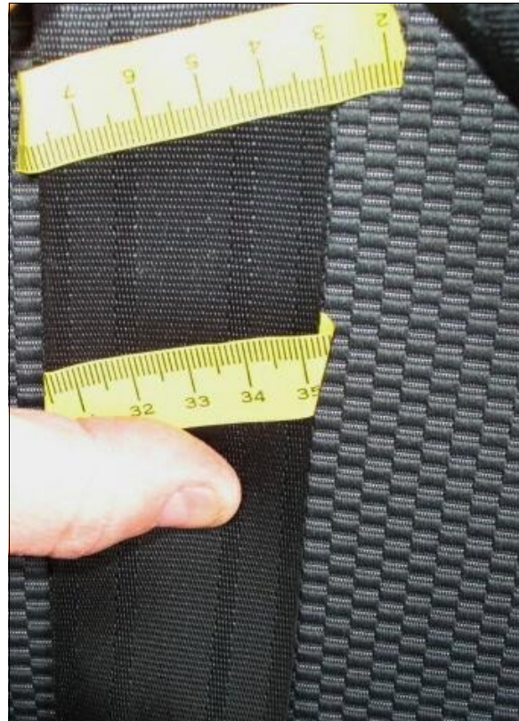
Figure 12: Loading evidence (faint scuff) on webbing of Mazda’s second row left safety belt
