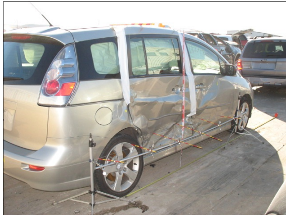
Figure 5: Mazda's right side damage viewed from back; C 1 begins behind right rear wheel
