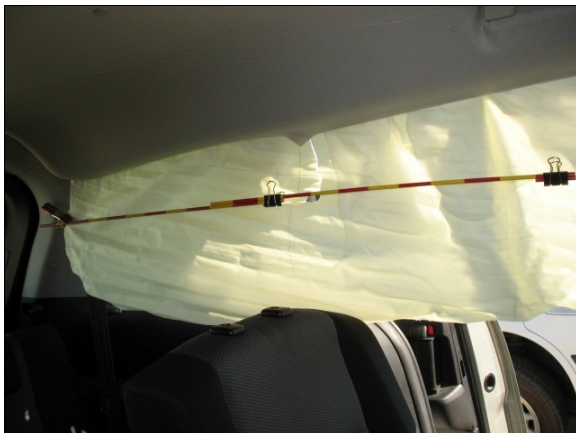
Figure 17: Back portion of Mazda's left side curtain air bag
