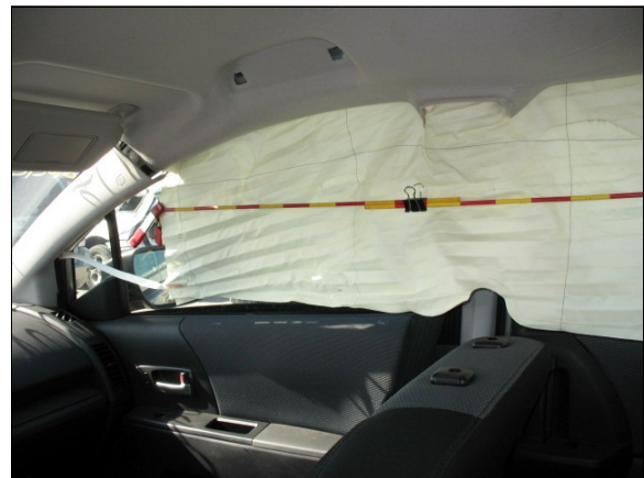
Figure 18: Front portion of Mazda's right side curtain air bag; tether attached to lower portion of right A-pillar
