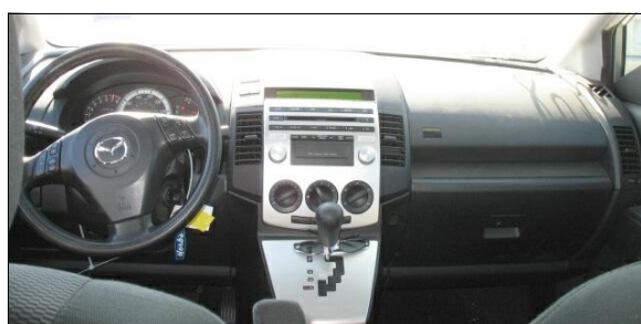
Figure 8: Mazda's instrument panel, steering wheel, and transmission selector lever with no apparent evidence of occupant contact, and non-deployed driver and front right passenger air bags
