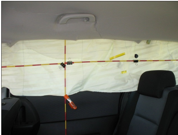
Figure 19: Middle portion of Mazda's right side curtain air bag; probable deployment scuff (upper and lower portions bracketed by tape) near second row right seat back
