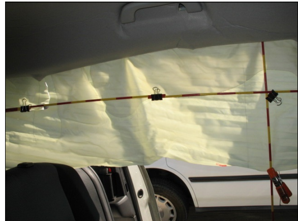
Figure 16: Middle portion of Mazda's left side curtain air bag
