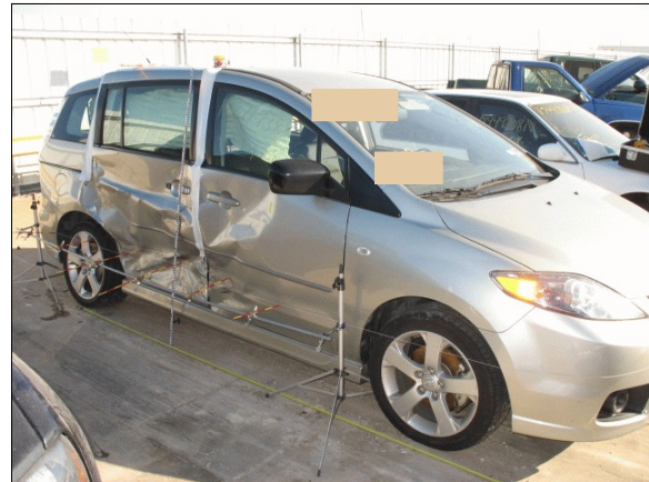
Figure 6: Mazda's right side damage viewed from front; C 6 located mid-right front door
