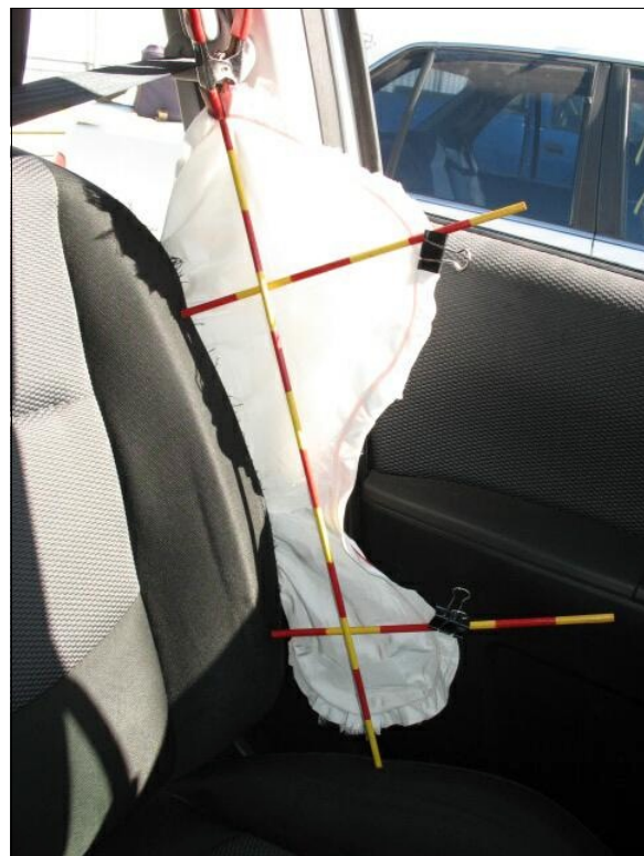
Figure 14: Inboard surface of Mazda’s driver seat back-mounted side impact air bag; no evidence of occupant contact was readily apparent
