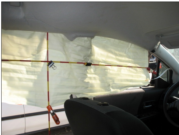
Figure 15: Front portion of Mazda's left side curtain air bag; tether attached to lower left A-pillar
