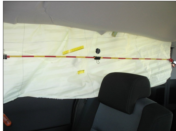
Figure 20: Back portion of Mazda's right side curtain air bag with probable deployment scuff bracketed by tape
