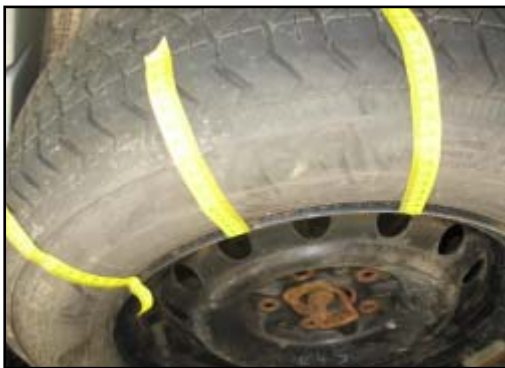
Figure 13. Contact to the rear aspect of the spare tire.
