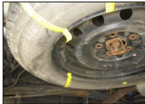
Figure 14. Area of contact to the left side of the spare tire.
