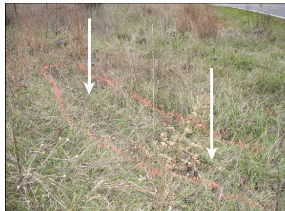
Figure 7: Impression on the ground where left portion of roof and left roof side rail touched down during second quarter turn; left arrow shows area of tempered glass fragments from left front window; right arrow shows area of tinted, tempered glass fragments from left rear window
