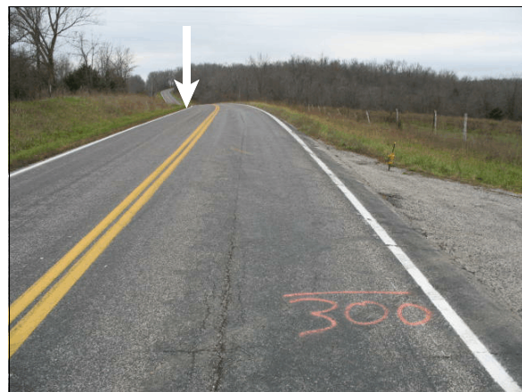
Figure 2: Southbound approach of the Chevrolet; number on pavement shows feet to area roadway departure to the rollover (arrow)
