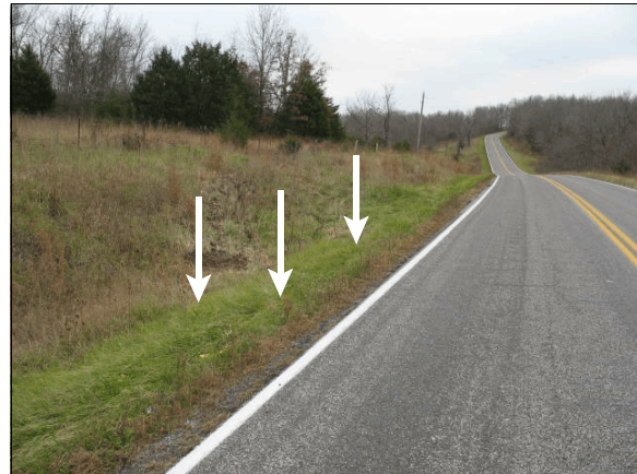
Figure 3: Chevrolet's approach to departure of east side of roadway with arrows (left to right) showing left front tire mark, right front tire mark, and right rear tire mark
