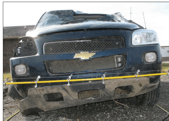
Figure 4: Damage to lower portion of Chevrolet's front bumper from impact with the embankment
