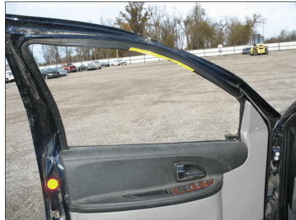
Figure 12: Driver was ejected out of left front window; yellow tape shows location of hair deposited in the window track
