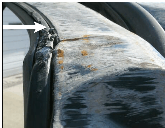
Figure 3: Front to rear view of top of right front door; arrow shows direction abrasions were formed
