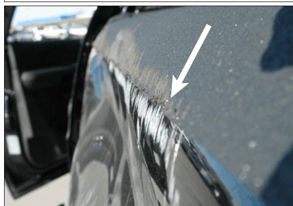
Figure 4: Arrow shows direction that abrasions were formed on the left side of the truck bed based on displacement of the bed liner material; view from back
