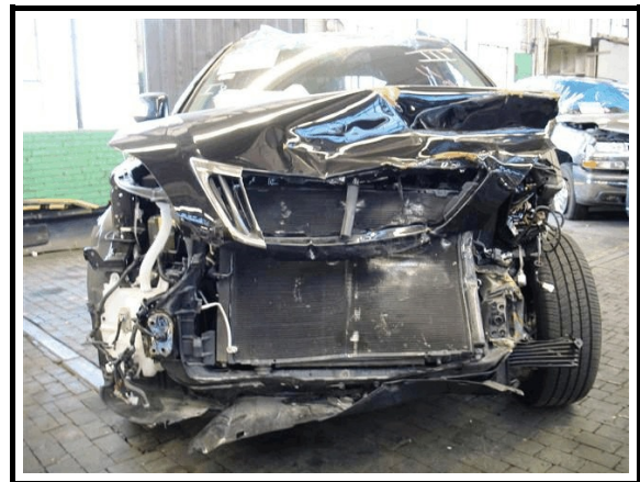
Figure 4. Front end damage, subject vehicle
