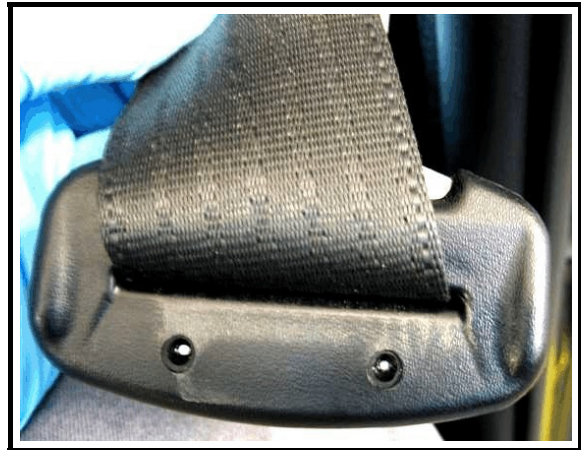
Figure 5. Abraded latch plate, driver's safety belt
