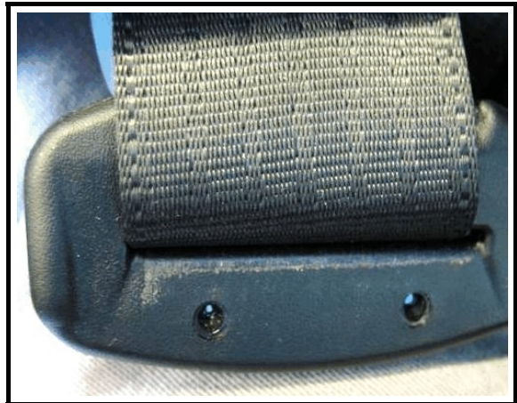
Figure 6. Abraded latch plate, front right occupant's safety belt
