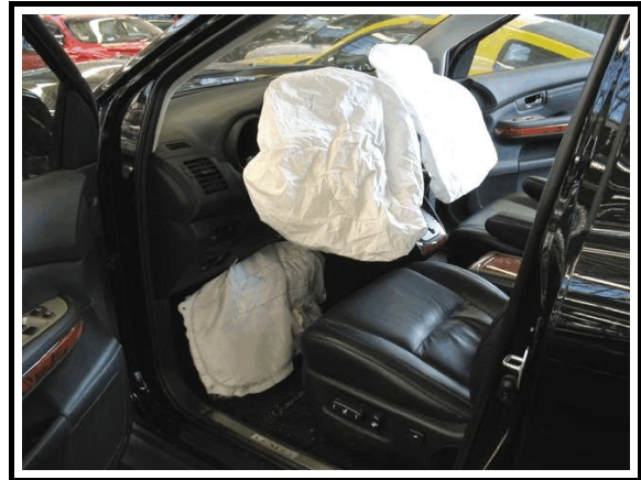
Figure 7. Deployed frontal and knee air bags
