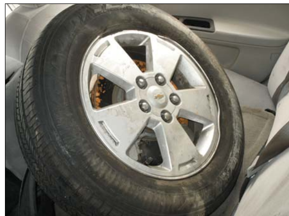
Figure 4: Left front wheel damage from curb impacts
