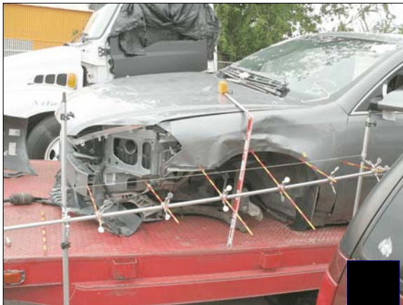
Figure 8: Damage to the left fender
