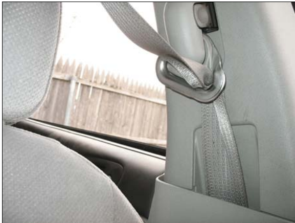
Figure 13: Driver's seat belt webbing wedged in D-ring
