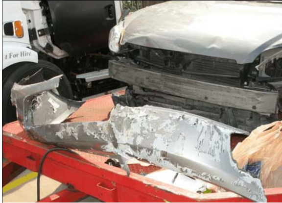
Figure 6: Damage to the front and front bumper fascia
