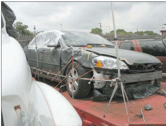
Figure 10: Right side damage
