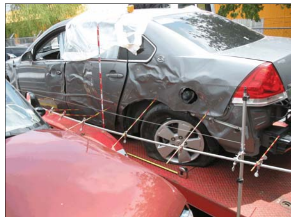
Figure 9: Damage to left side doors and quarter panel
