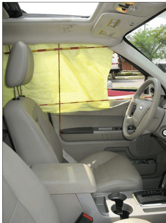
Figure 15: Gap between front of side curtain air bag and left A-pillar
