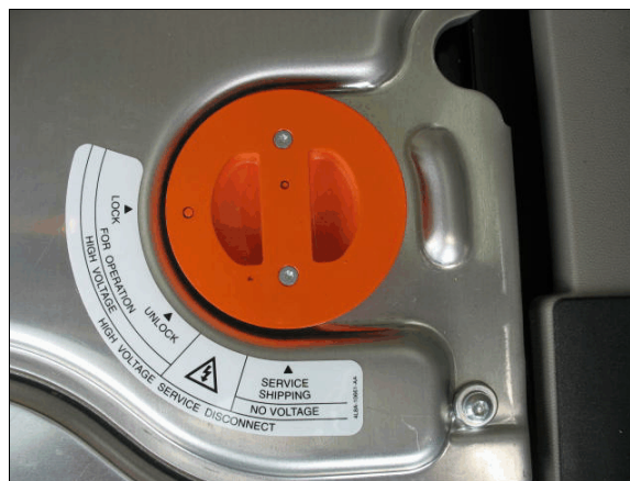
Figure 10: The high voltage service disconnect switch; switch in the locked position at the inspection
