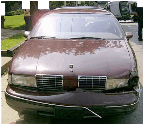
Figure 4: Damage to the front of the Oldsmobile from the impact with the Ford
