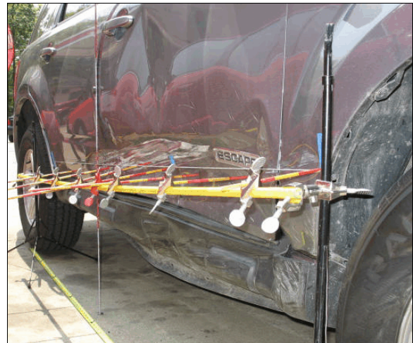
Figure 5: Damage to right side of Ford from impact by front of Oldsmobile
