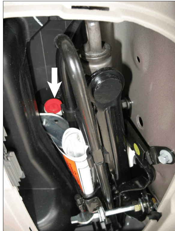
Figure 13: Arrow shows the inertia activated high voltage shut off switch located in the jack compartment
