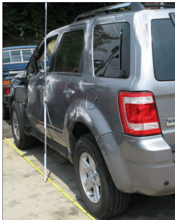
Figure 7: Damage to Ford's left side from the rollover
