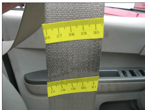
Figure 16: Plastic transfer from the sliding latch plate on the driver's seat belt webbing
