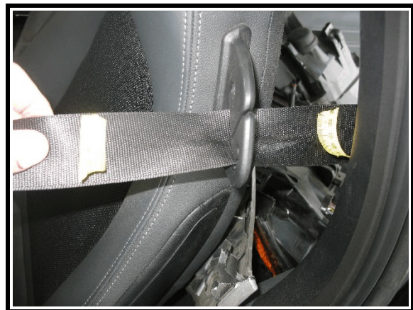
Figure 7. Loading to driver's seat belt webbing
