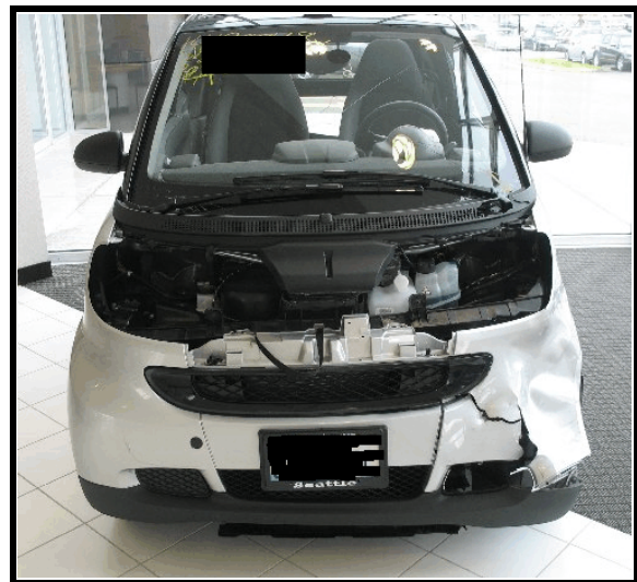
Figure 4. Frontal damage, 2008 Smart Fortwo
