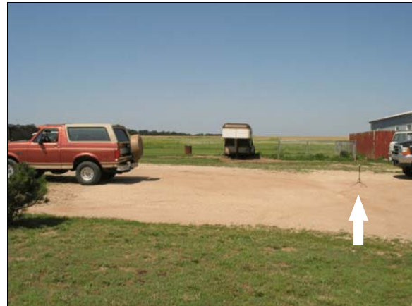
Figure 5: Arrow at target shows extent of blind zone with driver looking over shoulder
