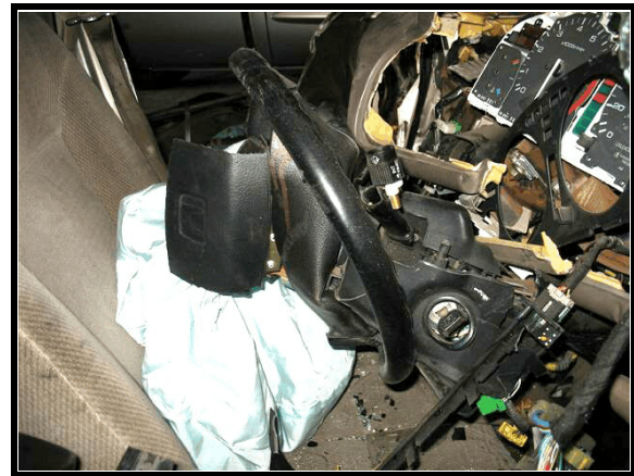
Figure 7. Intrusion and deformation of steering wheel and column
