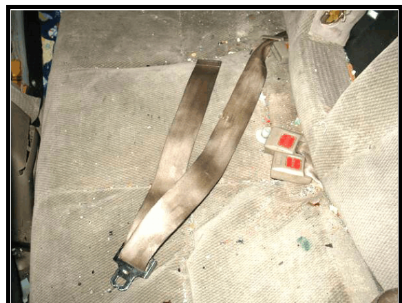
Figure 9. Second row center lap belt, used to secure a Baby Trend infant safety seat
