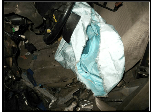
Figure 10. Driver's frontal air bag, showing tear down left side
