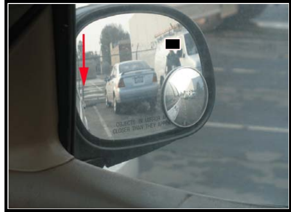
Figure 5. View through right side view mirror from driver's seat, arrow shows target where it begins to enter the mirror's lateral field of view (Note: convex mirror not present on subject vehicle)
