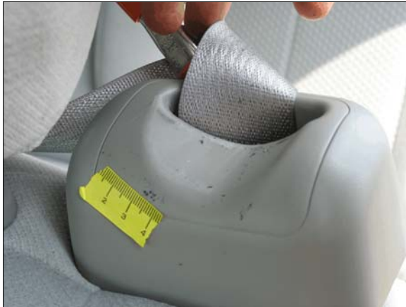
Figure 16: Load abrasions on driver’s seat belt housing
