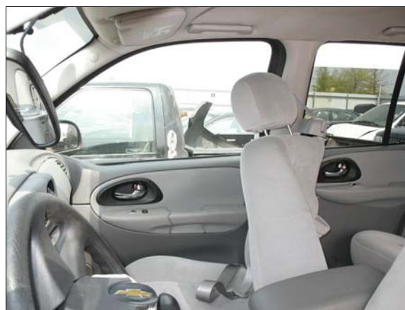
Figure 10: Deformation of the front right passenger seat back due to loading by the unrestrained second row right passenger
