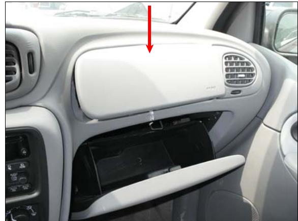
Figure 13: The front right passenger air bag module cover flap (arrow)
