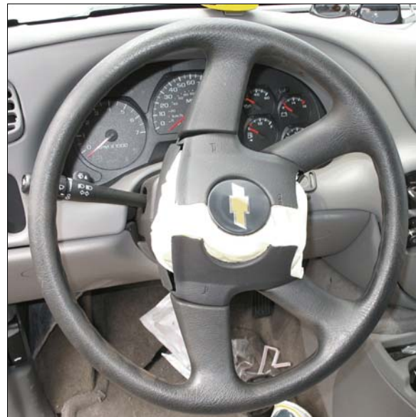
Figure 11: Driver's air bag module cover flaps; steering wheel rotated counterclockwise 90 degrees
