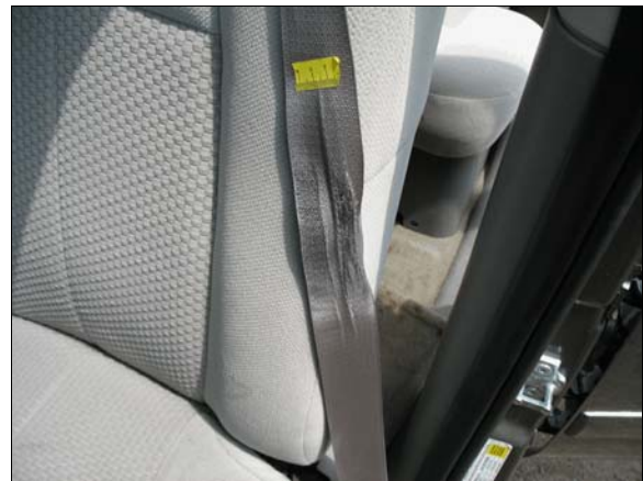
Figure 15: Load mark on driver's seat belt
