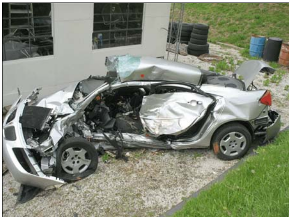
Figure 7: Damage to left side of Pontiac from impact with the Chevrolet
