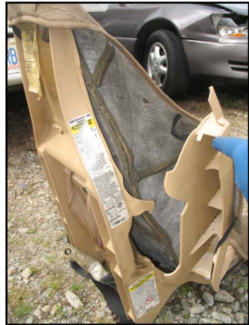
Figure 21: View of the right outboard fracture of the left CSS.
