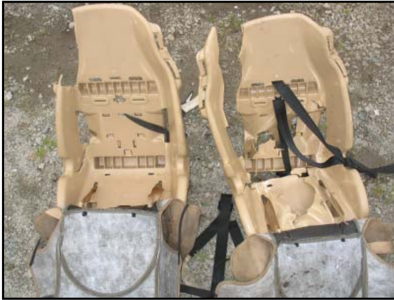
Figure 19: View of the fractured child safety seats.
