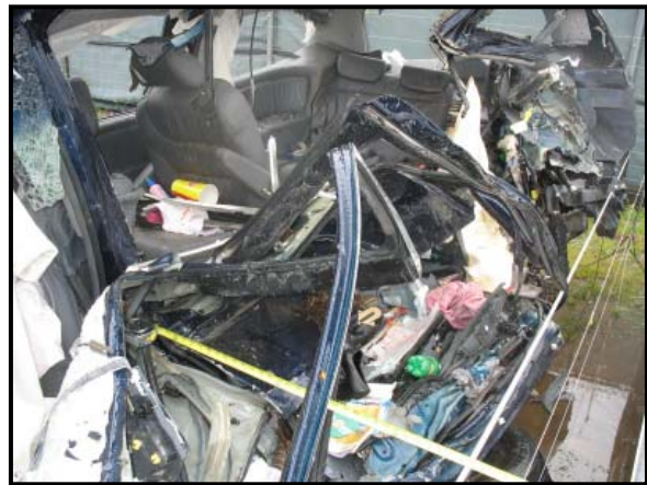
Figure 9: Left oblique view of the maximum crush at the B-pillar.
