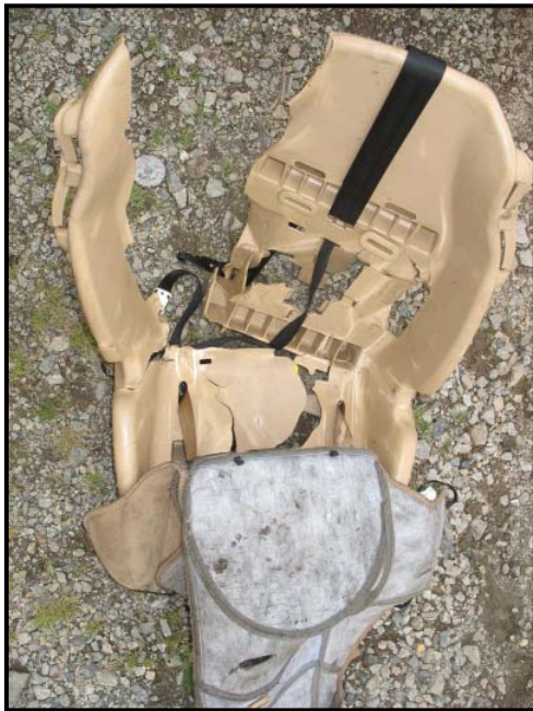
Figure 20: View of the complete fracturing of the right CSS.
