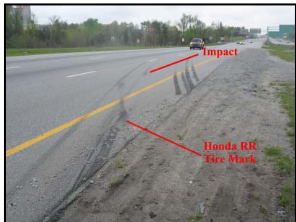
Figure 6: View of the POI and skid marks at the crash site.
