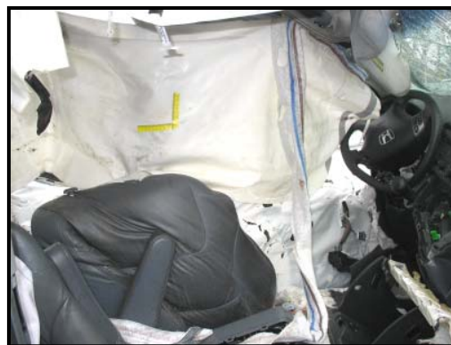
Figure 17: Possible driver contact to the left curtain.
