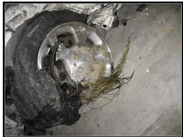
Figure 7. Left front tire/rim damage to Cherokee
