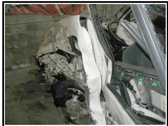
Figure 6. Left side damage to Cherokee
