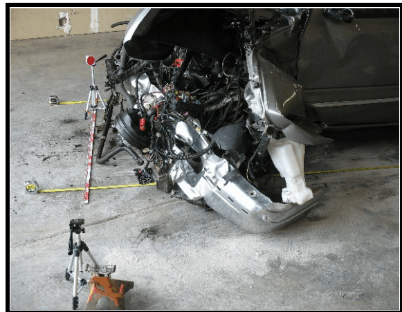
Figure 16. Side view of front end damage
