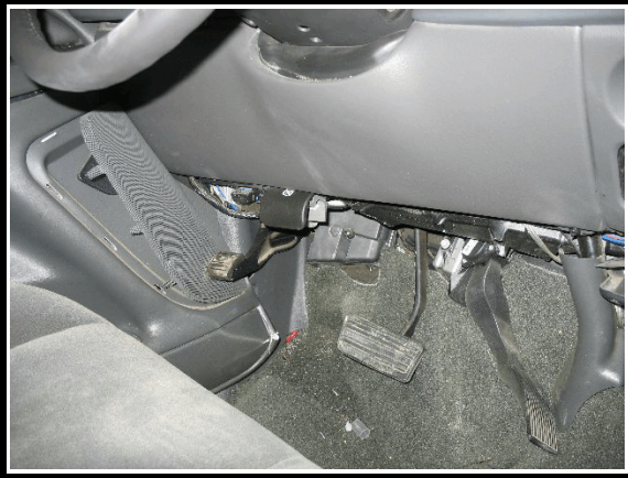
Figure 18. Left kick panel/toe pan intrusion
