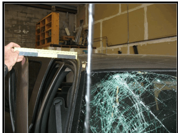
Figure 17. Front right door outward bowing
