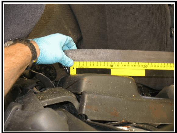
Figure 10. Second row left safety belt loading to belt webbing
