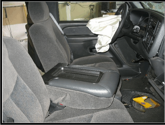
Figure 21. Side view of deployed driver's air bag
