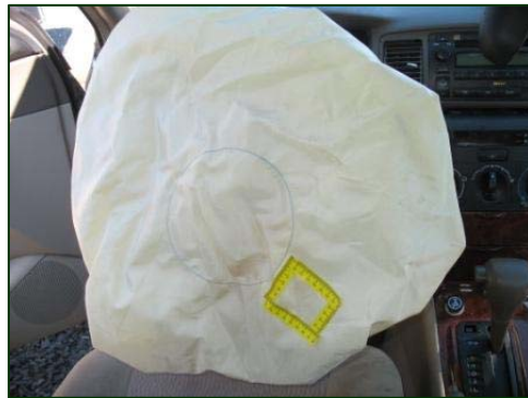
Figure 5. Deployed driver's air bag with make-up transfer.
