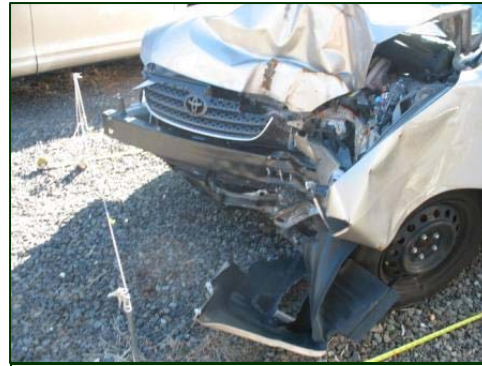
Figure 6. Lateral view of the depth of frontal crush.
