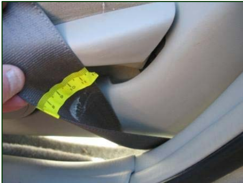
Figure 8. Lap belt transfer from recline lever.
