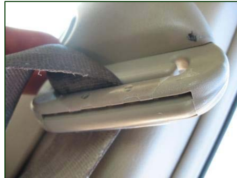
Figure 9. D-ring abrasion and belt evidence.
