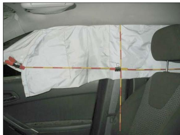
**Figure 10:** Front portion of right side curtain air bag; each increment on rods is 5 cm (2 in)
