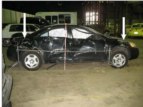
**Figure 3:** Damage to right side doors from contact with impact attenuator; left arrow shows damage from impact with concrete traffic barrier; right arrow shows damage to right fender from the rollover
