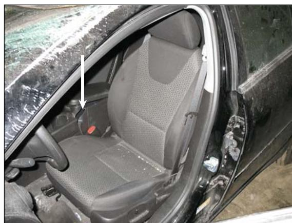
**Figure 8:** View of driver's seat and broken floor console (arrow)
