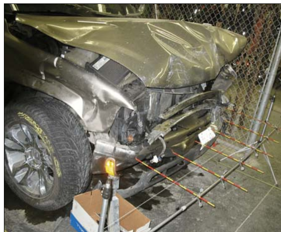
Figure 4: Front right view of damage to front of Chevrolet due to impact with left side of Toyota; each stripe on rods in 5 cm (2 in)
