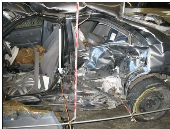
Figure 6: Arrow shows location of maximum crush; vertical scale is graduated in meters and tenths of meter
