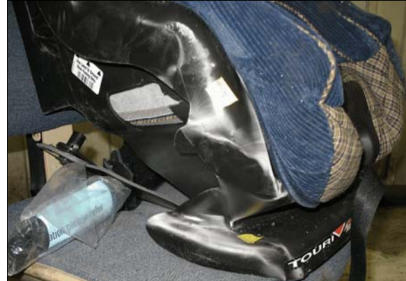
Figure 10: Damage to base and right side of child safety seat
