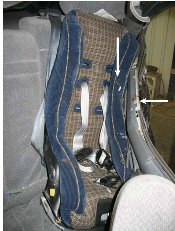
Figure 7: Cosco Touriva CSS entrapped in Toyota's back left seat position; left arrow shows blood and tissue transfer on left side surface of CSS; right arrow shows blood and scuff marks on left rear window sill
