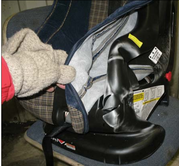
Figure 9: Damage to left side of child safety seat
