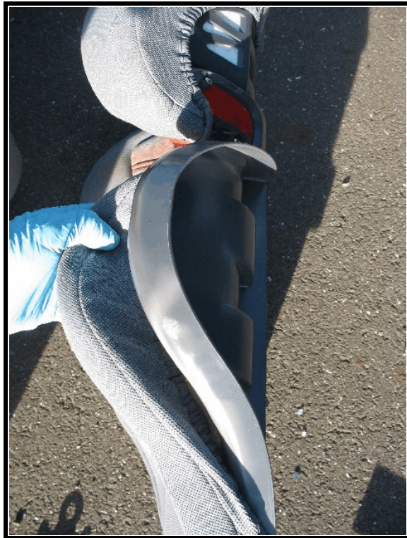
Figure 14. Cracking to left seat back
