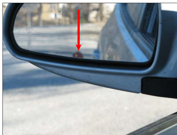
Figure 9: Close view through Hyundai’s left side view mirror; arrow shows target at location it began to go out of driver’s view as it was moved forward from back left bumper corner
