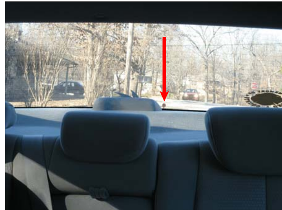
Figure 7: View out of Hyundai's backlight from driver's seat; arrow shows target in location where driver could first see it
