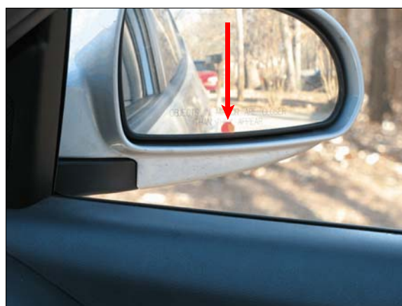
Figure 10: Close view through Hyundai’s right side view mirror from driver’s seat, arrow shows target at location it began to go out of driver’s view as it was moved forward from the back right bumper corner
