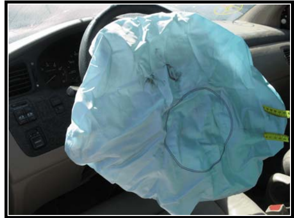
Figure 6. Deployed driver's air bag
