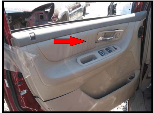
Figure 8. Possible contact to door panel
