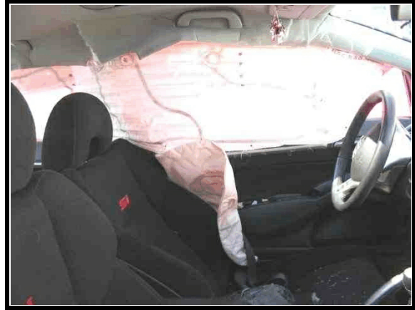
Figure 6. Driver's side curtain air bag and seat mounted side air bag
