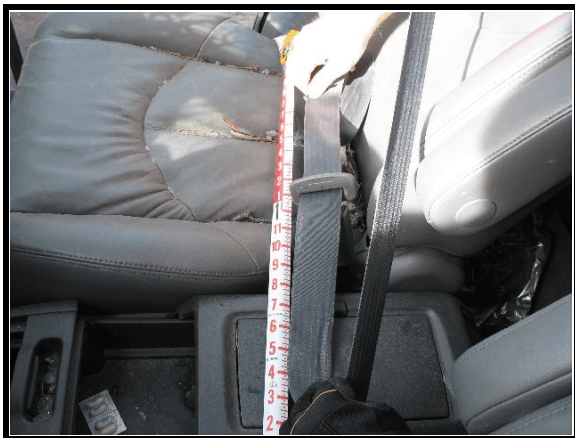
Figure 13. Loading to front right passenger seat belt webbing
