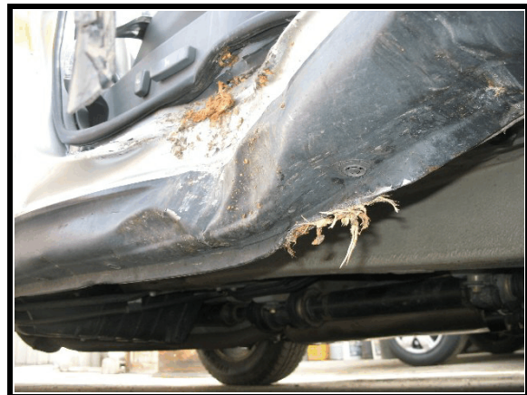
Figure 18. Right side impact damage
