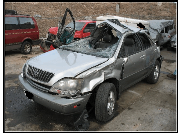
Figure 6. Left side damage, Lexus RX300
