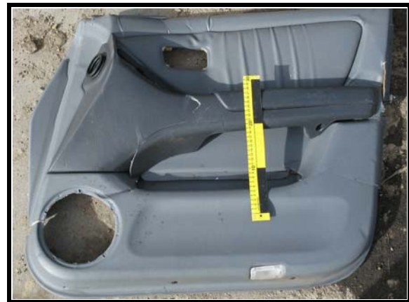
Figure 19. Contact to interior door panel/armrest
