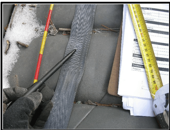
Figure 15. Missing stop button on front right passenger seat belt
