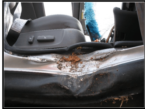
Figure 9. Close up of right sill damage
