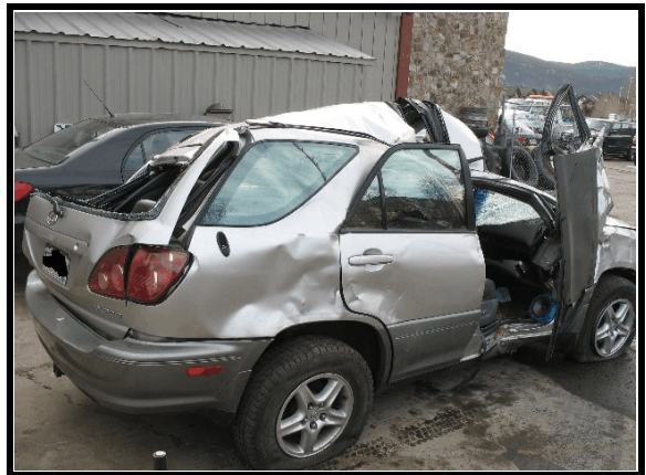
Figure 7. Right side damage, Lexus RX300
