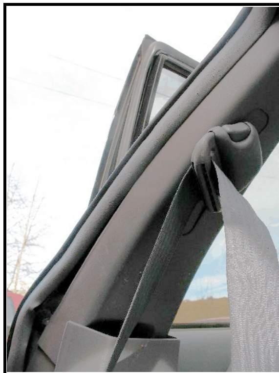
Figure 16. Front right seat belt D ring position
