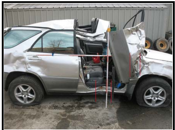
Figure 8. Right side tree damage
