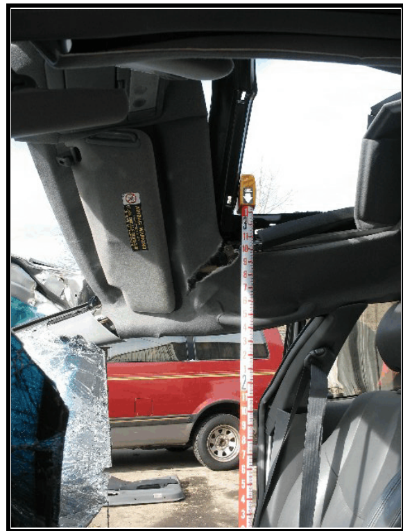
Figure 10. Right roof rail and A pillar intrusion
