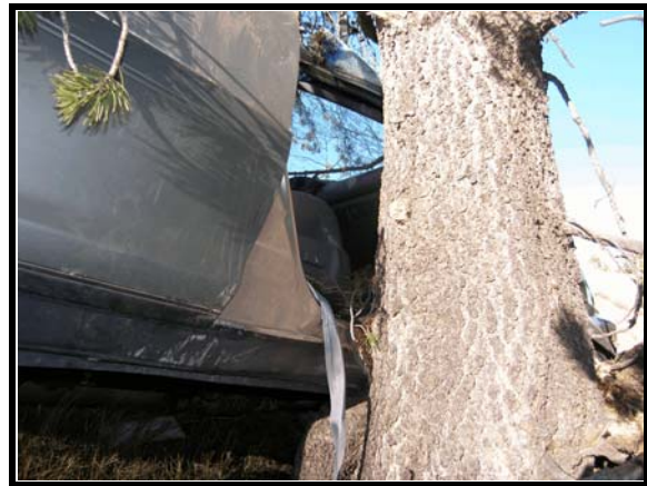
Figure 5. Right side of Lexus RX300 at tree contact
