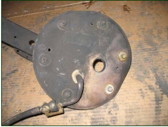
Figure 19: Deformation to the sending unit.
