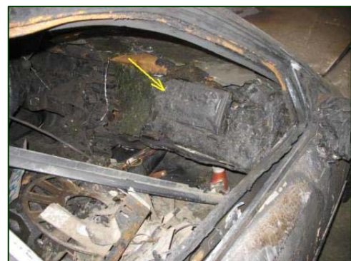
Figure 13: Non-deployed front right air bag.
