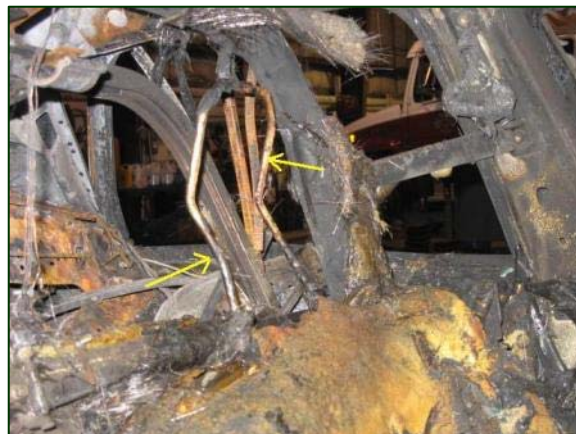
Figure 22: Driver loading deformation of the head restraint frame.
