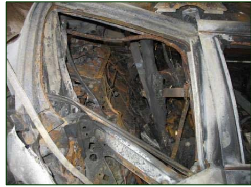
Figure 11: Intrusion of the right rear seat position.
