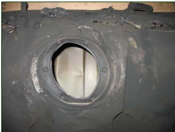
Figure 17: Deformed sending unit port.
