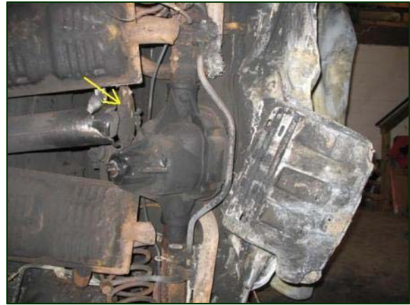
Figure 15: Separated fuel pump/sending unit.
