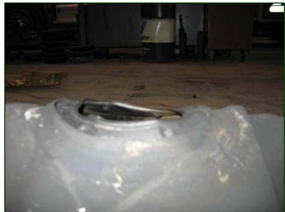
Figure 18: View across the deformation of the sending unit port.
