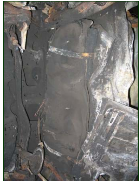
Figure 16: Fuel tank with surrounding components removed.
