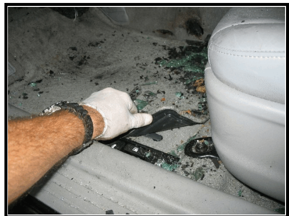
Figure 31. Carpet mat and left mat retention device
