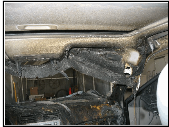
Figure 11. Right A pillar/header scorching damage
