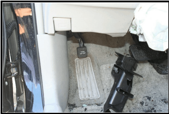
Figure 26. Parking brake in full down position (as found at scene)
