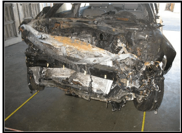
Figure 8. Frontal damage from impacts with two vehicles
