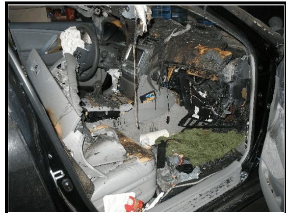
Figure 9. Right instrument panel damage
