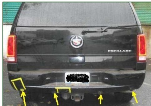
Figure 12. Rear ultrasonic sensors.
