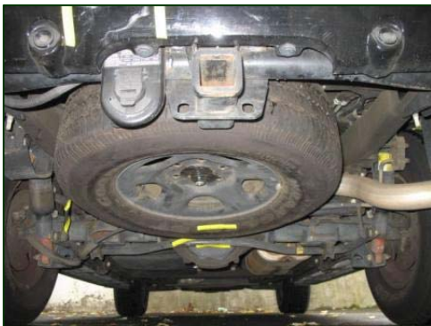
Figure 10. Wipe marks to the spare tire and rear sway bar.
