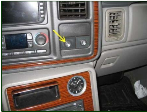
Figure 13. Position of the URPA switch.
