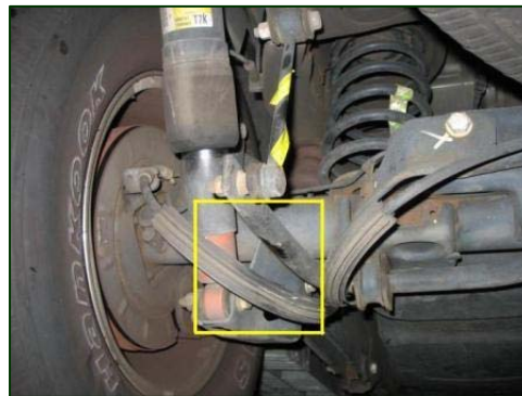
Figure 11. Wipe marks to the sway bar, stabilizer and emergency brake cable.
