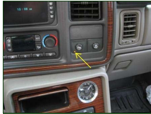
Figure 14. URPA switch OFF indicator light.
