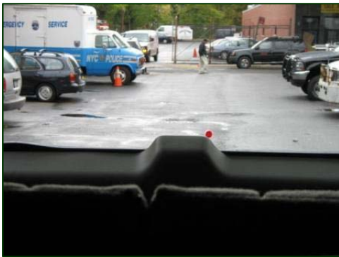
Figure 16. Red reflective target visible through centerline of backlight.
