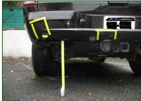
Figure 9. Suspected contact evidence to the back bumper fascia.
