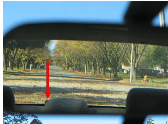
Figure 9: Close view of target (arrow) on left side of CHMSL as seen through rearview mirror viewed from driver's seat
