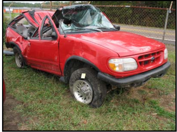
Figure 5: Front right oblique view of the Ford. 14 cm (5.5 in) of induced vertical crush as a result of the roof impact. This area began 3 cm (1 in) forward of the right rear axle.
