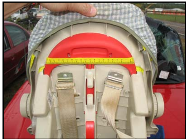
Figure 13: Back view of the fractured shell.
