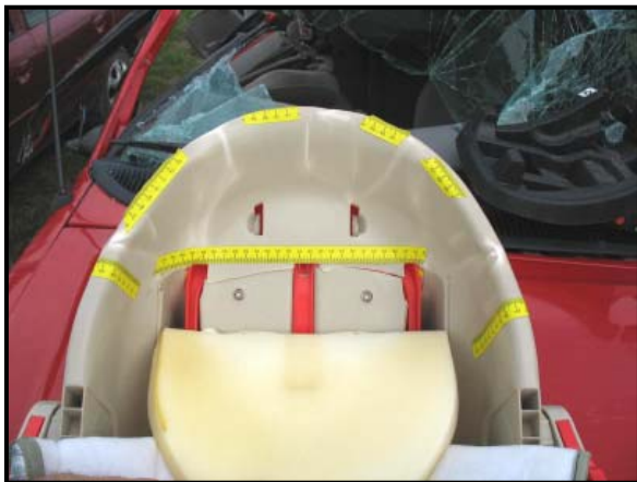
Figure 12: Stress marks and fracture across the arch of the upper shell
