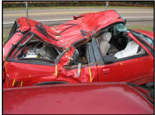
Figure 6: Right side view depicting the roof deformation.
