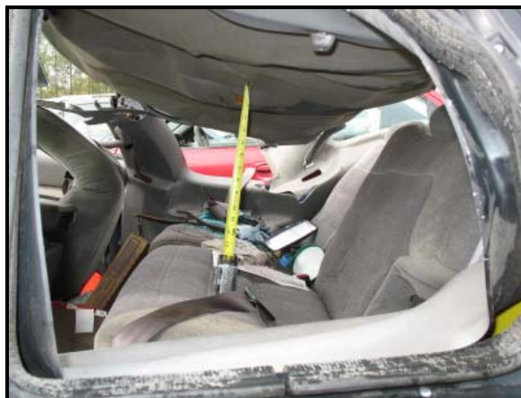
Figure 7: Measurement of the residual roof height above the left rear seat cushion.
