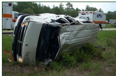
Figure 13. Rollover damage to the Dodge B350 van.
