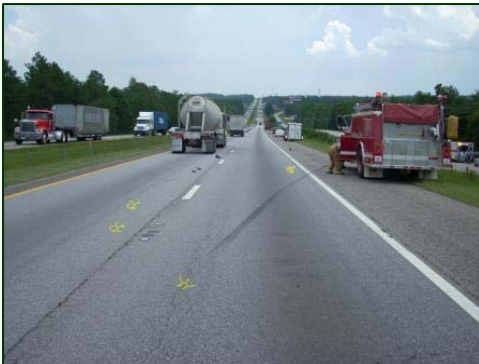
Figure 11. CW yaw marks on the travel lanes of the interstate.
