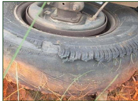
Figure 10. Close-up view of the remaining tire carcass and inner steel belt.
