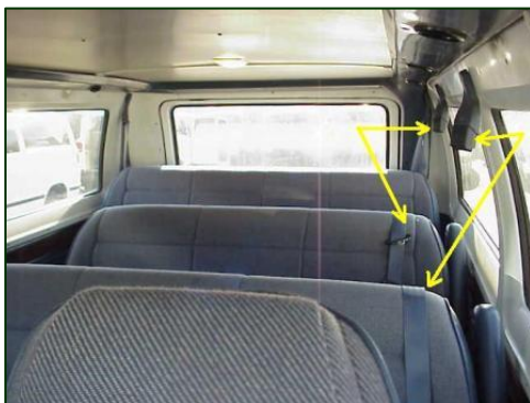
Figure 14. Detachable left side shoulder belts of an exemplar vehicle.
