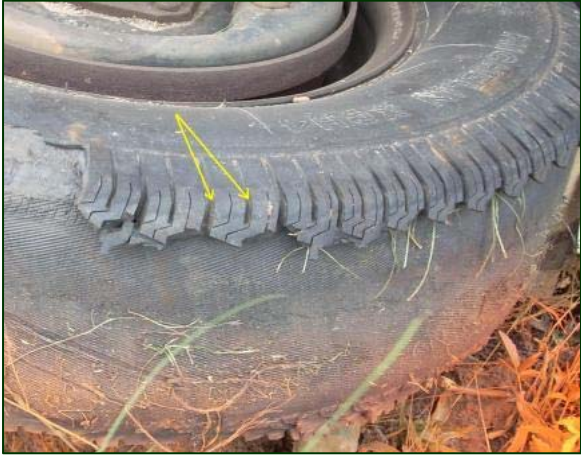
Figure 6. Edge of the remaining tread of the left rear tire.
