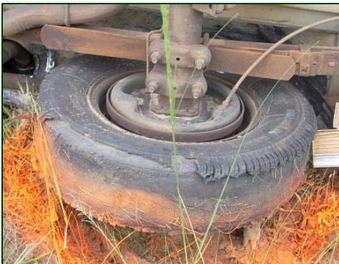
Figure 9. Tire tread separated from the left rear tire.
