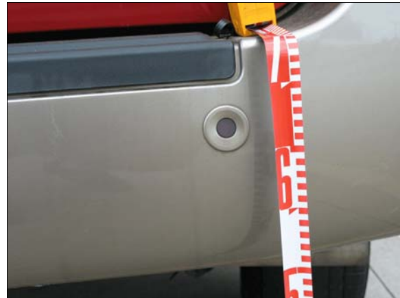
Figure 5: Closeup of reverse sensor near back right bumper corner, scale in tenths of meter, end of scale on ground
