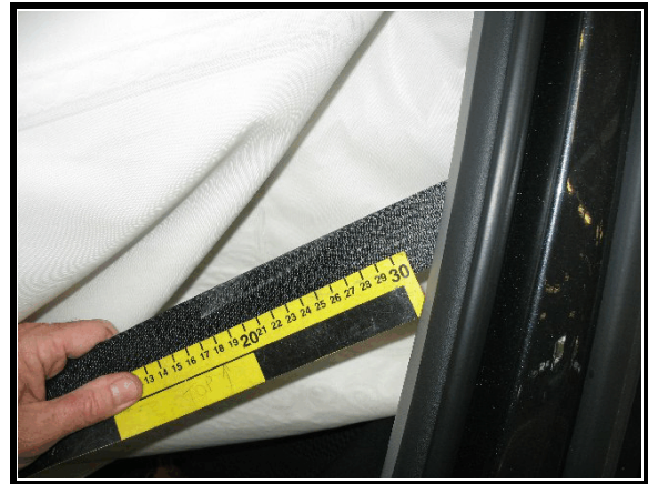
Figure 9. Load marks to driver's seat belt webbing
