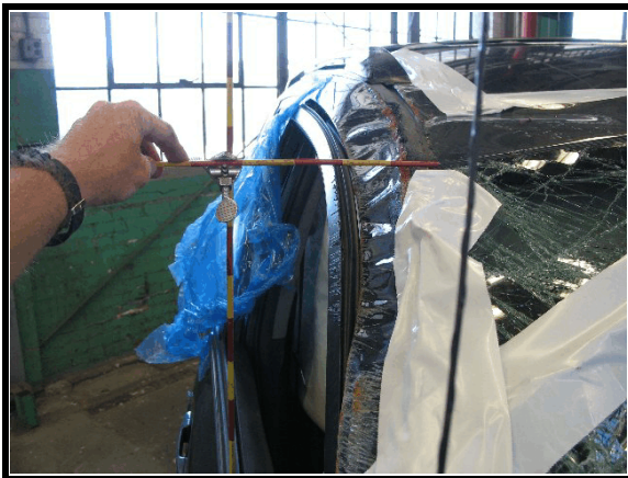
Figure 8. Maximum crush at right A pillar area
