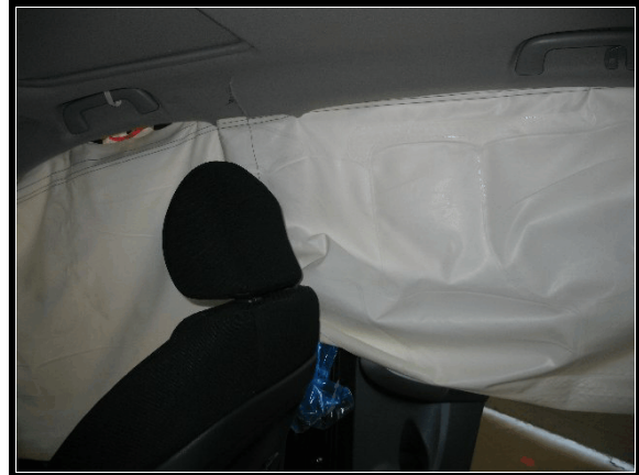
Figure 11. Front right passenger side air curtain
