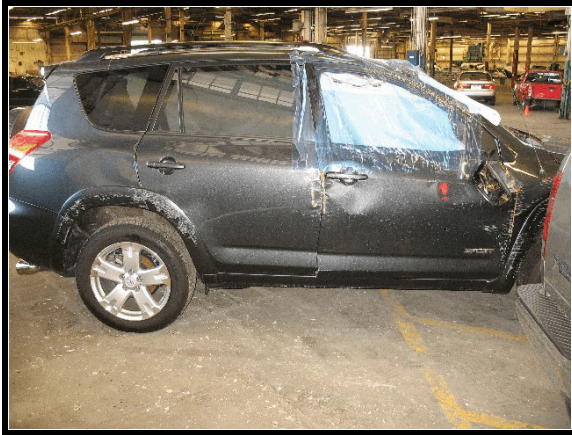
Figure 6. Right side rollover damage
