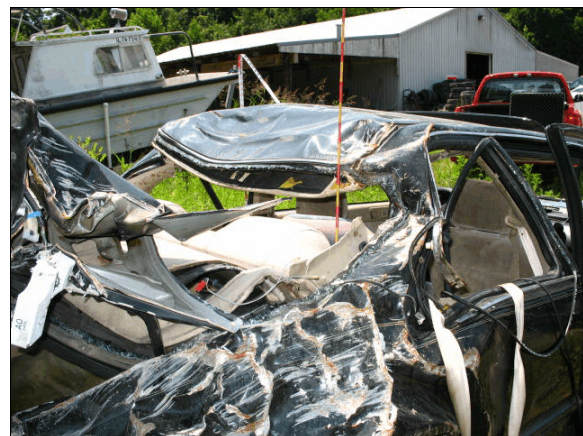
Figure 6: Overview of crush to the Honda’s roof, backlite header and right C-pillar; each increment on the measurement rod is 5 cm (2 in)
