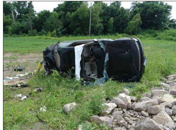
Figure 5: Sheriff department’s on-scene photo of Honda’s final rest; windshield cut out by rescue to extricate front right passenger
