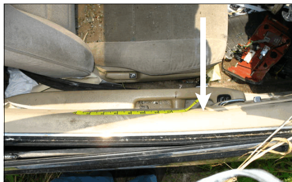
Figure 11: Right front door slightly bowed outward from contact by front right passenger
