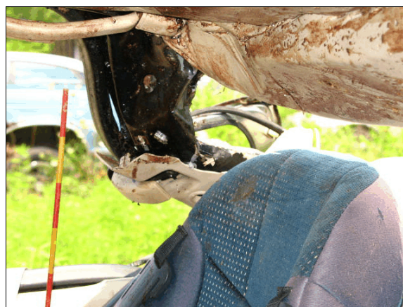
Figure 12: The second row right passenger contacted his head on the intruded right C-pillar
