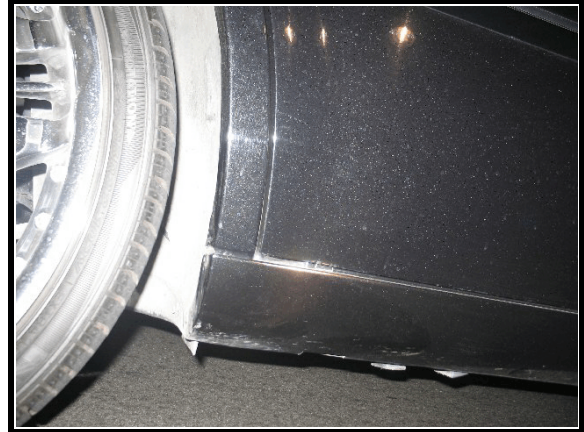
Figure 11. Scuffing to area forward of right rear tire
