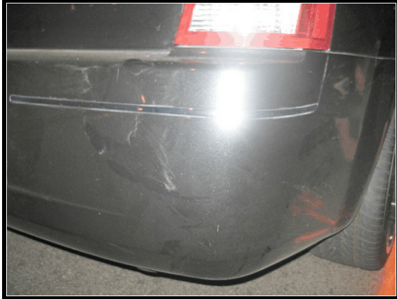
Figure 10. Scuffing to right rear bumper
