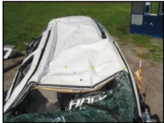
Figure 6: View of the roof deformation.
