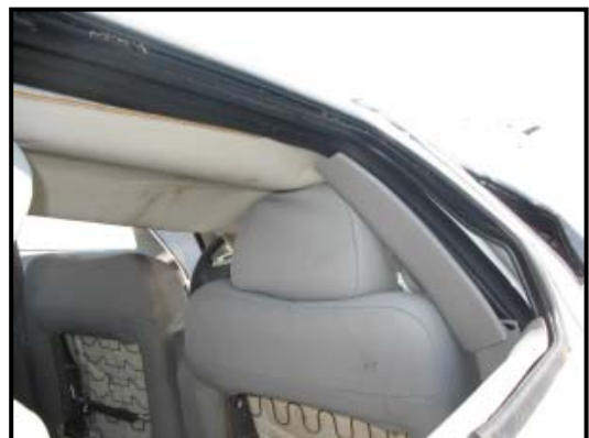
Figure 7: View of the front right seat back and intrusion.
