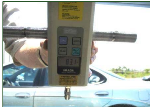
Figure 4. Peak closing force reading of 370 N (83.1 lbs) of the rear right power window.
