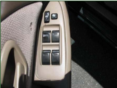
Figure 3. Driver's power switch console on an exemplar vehicle.
