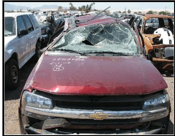
Figure 3. Overview of roof crush as seen from the front of the vehicle
