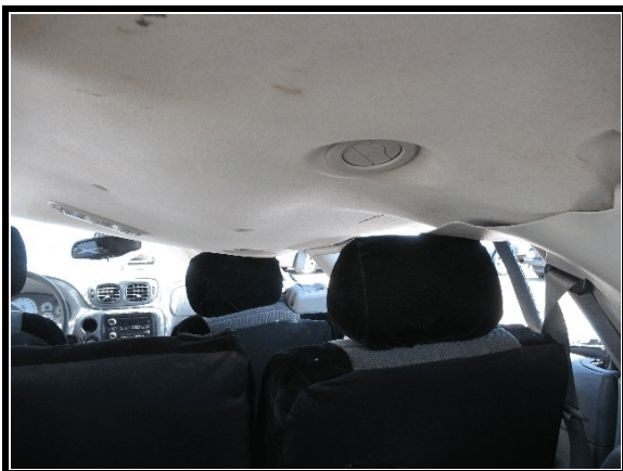
Figure 5. Overview of right side intrusion
