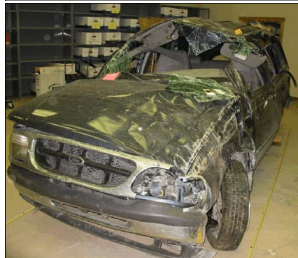
Figure 2: Front left view of rollover damage to the Ford. The left side pillars had been cut by rescue personnel, and the roof crush was altered during rescue operations.
