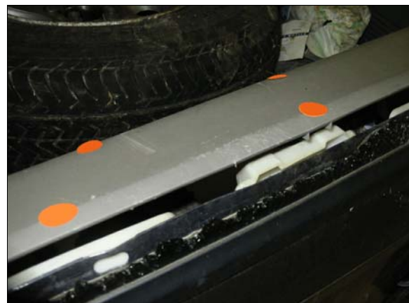
Figure 7: Abrasions (outlined by orange dots) located on the left window sill in Ford's cargo area.
