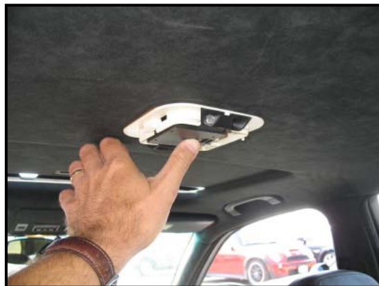
Figure 6: Center roof mounted sensor (exemplar BMW).
