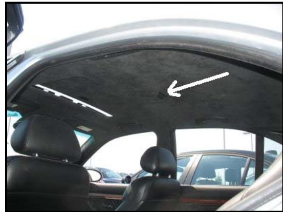
Figure 5: Center roof mounted interior motion sensor in an exemplar BMW M5.
