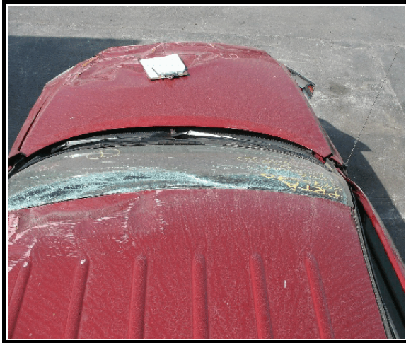
Figure 6. Roof and hood damage
