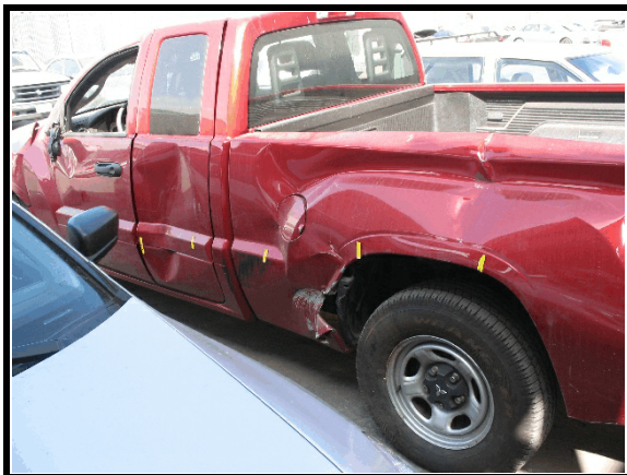
Figure 3. Left side damage, impact 1
