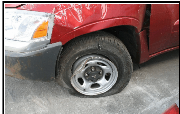
Figure 4. Tire/rim damage, impact 2
