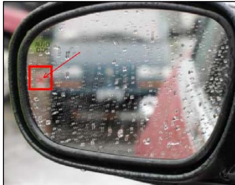
Figure 11. Visible red target in left outside rear view mirror.
