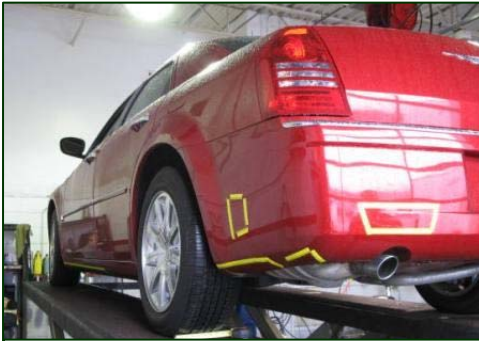
Figure 8. Contact evidence (wipe marks) to the left side surface of the rear bumper fascia.
