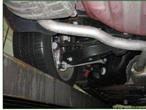
Figure 7. Left rear muffler and suspension components.
