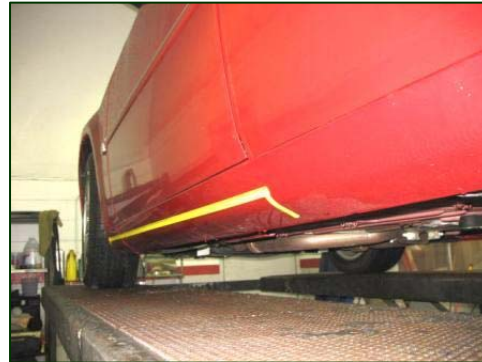
Figure 9. Left lower sill wipe marks.
