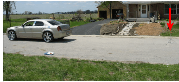
Figure 7: Arrow shows location target first came into view while surrogate driver was looking over right shoulder through gap between center high-mounted brake lamp and back left head restraint.
