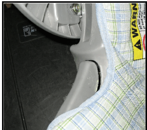
Figure 9. Scuffing, right seat belt guide 6
