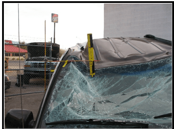
Figure 9. Front view of roof damage
