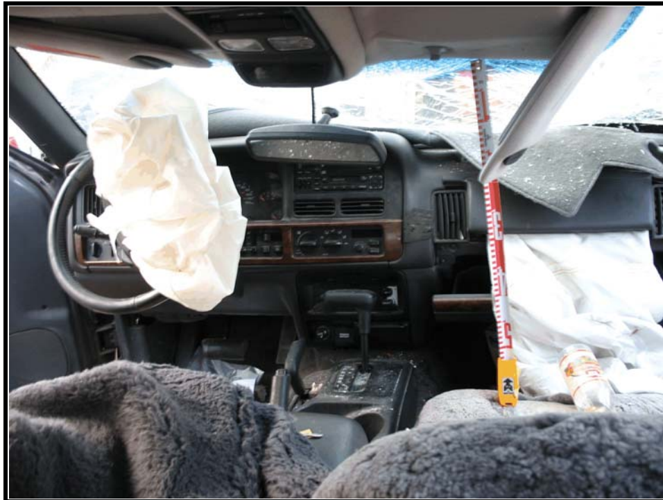
Figure 10. Overview of roof/windshield header intrusion
