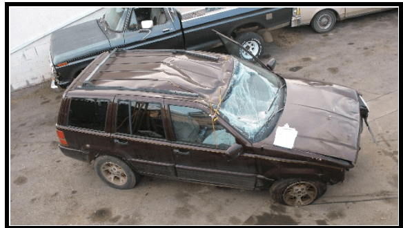
Figure 8. Top view of roof damage
