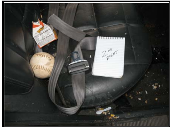
Figure 12. Cut section of second row right seat belt webbing
