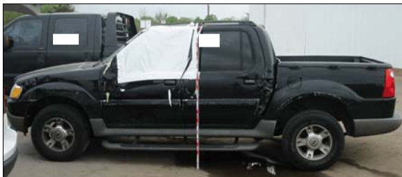
Figure 4: Overview of minor rollover damage to left side of
