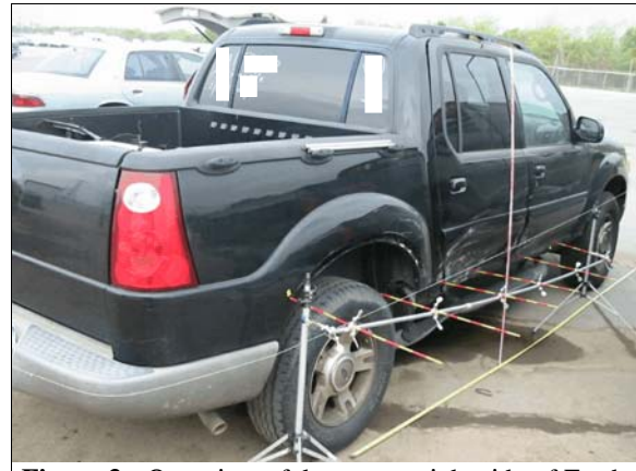
Figure 3: Overview of damage to right side of Ford due to impact with the Nissan
